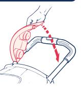
• Rotate down to opposite side and snap in place.
